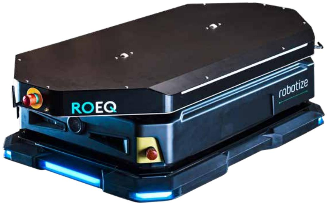
The ROEQ TMC300 top module is designed for the Robotize GoPal P35 to transport the ROEQ Cart500. With this cart solution the Robotize GoPal P35 can safely pick up, transport and drop off cargo of up to 300kg.
